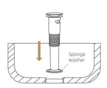
Put the lock nut inside the drainer body and screw on the nut tightly.
